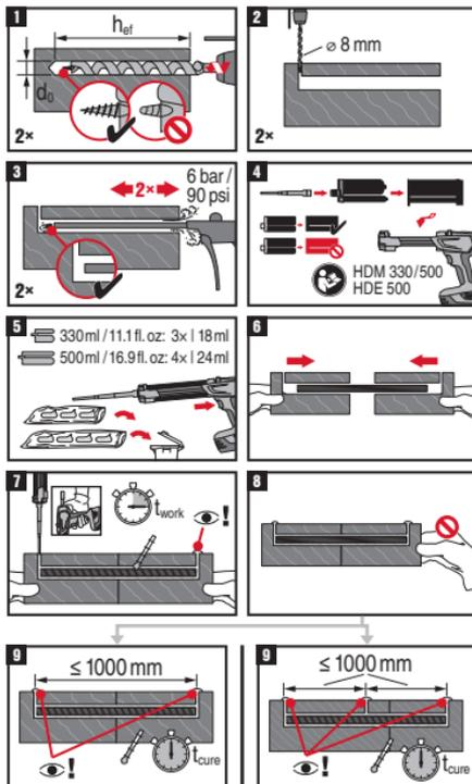
**EN Adhesive anchoring system for rebar and anchor fastenings in concrete/wood****Hilti HIT-RE 500 V4**
